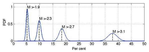
Figure 5: Probability distributions of percentage of nodes in the grid domain with simulated magnitudes above a specified value.
