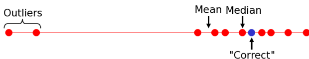
Figure 1: The arithmetic mean is skewed by outliers, while robust estimators like the median give a reasonable answer.
