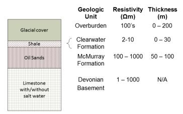
Figure 1: Typical geological section and related resistivity properties for the Fort McMurray area, Alberta.
