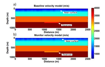
Figure 2: Earth model representing baseline model (a) and monitoring model (b). Both models have different near-surface and reservoir layer velocities. GeoConvention 2012: Vision
