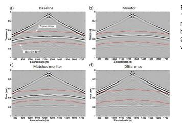
Figure 3: An example of a shot gather at x-coordinate 1250m from baseline survey (a), monitoring survey (b), matched monitoring survey (c) and the difference (d) between the baseline shot and the matched monitoring shot. The NRMS of the difference is shown in (e). The window of analysis is between the two red lines.
