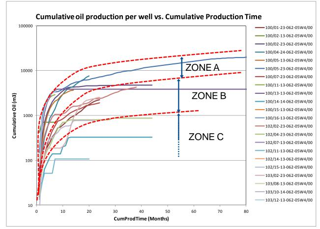
Figure 5. Cumulative oil production vs. cumulative production time for 22 wells, identifying 3 zones.
