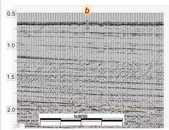
Left - Numerous diffractions associated with this probable hydrocarbon sourced seafloor feature are present on this unmigrated seismic section at ~1.2 seconds. Hydrate formation may not have occurred here due to the highly faulted nature of the section as indicated by the many diffractions which would allow leakage. Note the rapid drop in seismic reflectivity to the right of the feature at **b**.
