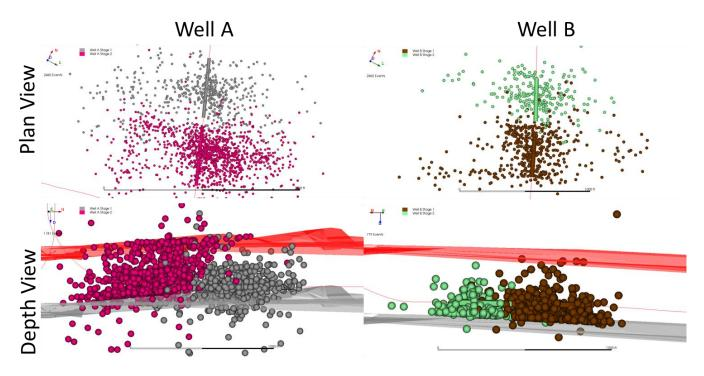
Figure 1: Events from 4 stages (2 in each well) shown in plan and cross-sectional view. The events are colourcoded by stage and shown for well A to the left and well B to the right. Also depicted is the top and bottom of the Marcellus as the red and grey surfaces.
