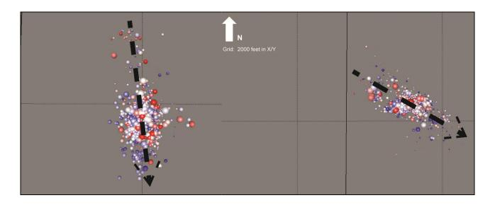
Figure 3: Observed microseismicity trends in the San Juan Basin of Rio Arriba County, NM. Well 1 (left) = 172° azimuth (Fracture Set I); Well 2 (right) = 130° azimuth (Fracture Set II).
