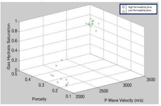
Figures 6a and 6b: 3D visualization of the correlation between gas hydrate NMR-derived gas hydrate saturation, P wave velocity and CMR Permeability computed using SDR model (Figure 6a) and density log-derived porosity (Figure 6b) for the high and low permeable zones of the Mallik 5L-38 well, shown in blue and green respectively.
