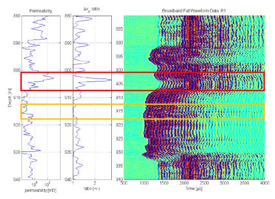
Figure 3: MRIderived permeability values, P-wave velocity dispersion ratio values (computed using the cross correlation method outlined in Pun et al) and broadband full waveform data recorded by receiver 1 in the Mallik 5L-38 research well. The areas of high and low velocity dispersion ratios are outlined in red and yellow respectively. (Based on Pun et al)
