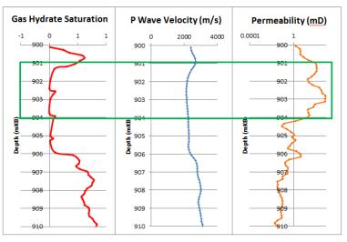
Figure 4: NRM-density log derived gas hydrate saturation, P wave velocity and CMR permeability computed using SDR model borehole logs for a high permeability zone of the Mallik 5L-38 well.
