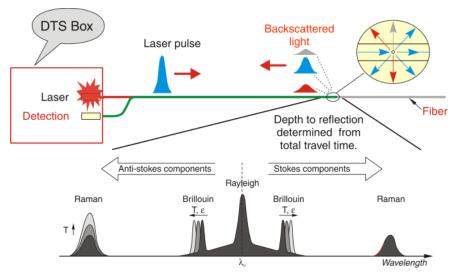
Fig. 1—DTS operating principle; Rayleigh backscatter.
