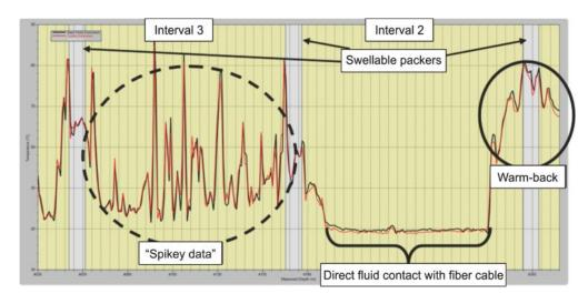
Fig. 2—DTS data acquired during stimulation of the openhole completion Interval 2.
