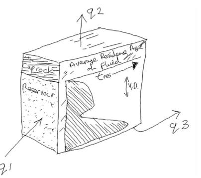
**Fig 2.** Schematic illustration of fluid fluxes (oil, gas, water, CO<sub>2</sub>) in and out of a reservoir. For example a charged flux of say, oil q1, contributes via storage and transport in the reservoir to leakage through the caprock-q2 and spillage from the spill point of the trap-q3. By age dating the fluid residence time profile in the reservoir and comparing it with radio nuclide distribution using a fluid age mixing model, in principle, the charge history and fluxes may be delimited.
