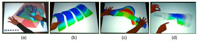
Figure 4: Depictions of our internal exploration techniques: (a) bounding box cut, (b) splitting, (c) peeling and (d) focus and context for wells.
