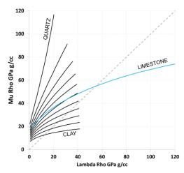
Figure 1. Rock-phsyics template in LMR for varying quartz-clay mixtures. Each line represents a 10% increase in quartz content from the clay line to the quartz line. A pure limestone trendline is also included (blue line). Note that porosity increases towards the origin.
