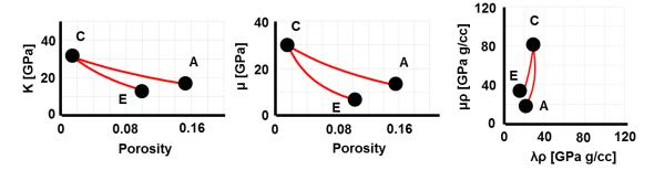
Figure 3. Bulk and shear modulus versus porosity in addition to an LMR crossplot showing bi-modal grain mixture rock physics templates. The points A, C and E refer to the grain geometries in Figure 2.
