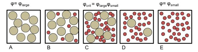
Figure 2. Large and small grain geometries used to model dispersive rock physics model implying rock texture and fabric. The critical porosity geometric configuration is when the pore space of the large grains is equal to the volume of the packed small grains (Figure 2C). When the pore space of the large grains is greater than the volume of the packed small grains, then small grains can reside with the large grain matrix (Figure 2A). This condition can be represented as:
