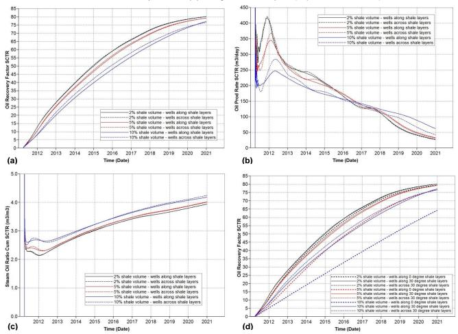
Figure 3: (**a**) oil recovery factor, (**b**) oil production rate, and (**c**) cumulative steam oil ratio versus time for 2, 5 and 10% shale volume with 30° dip and two well orientations, (**d**) comparison of oil recovery factors for models with zero and 30° dip angle shale layers
