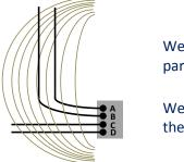
Well-pairs **A** and **B** are drilled parallel to the strike of the beds
