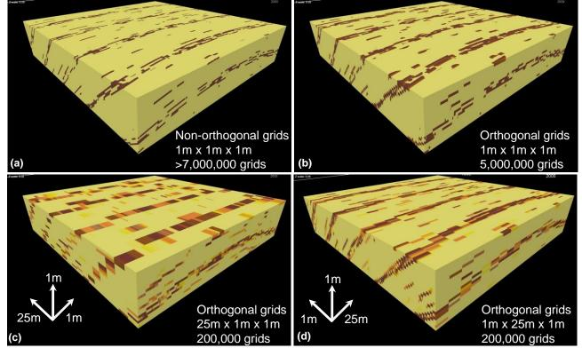
Figure 5: point bar models: **model (a)** using non-orthogonal and fine grids, **model (b)** using orthogonal, fine and rescaled grids, **model (c)** using orthogonal and up-scaled grids across the point bars, and **model (d)** using orthogonal and up-scaled grids along the point bars (aspect ratio: z/x=5/1).
