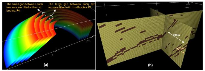
Figure 4: (**a**) circular arcs used for creating a point bar system, and (**b**) non-orthogonal grids used in geomodel for creating 3D inclined arc surfaces and mud bodies with 10° dip (aspect ratio: z/x=9/1).
