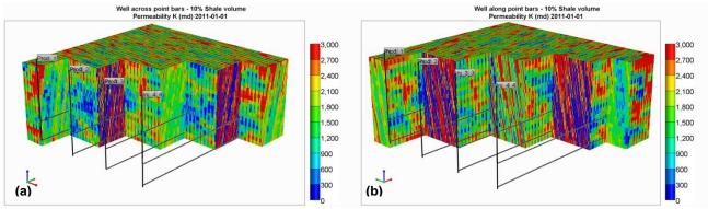
Figure 2: slab views of the vertical permeability distribution for the case of10% shale volume. Wells are placed (a) across the shale layers, and (b) along the shale layers (aspect ratio: z/x=9/1).
