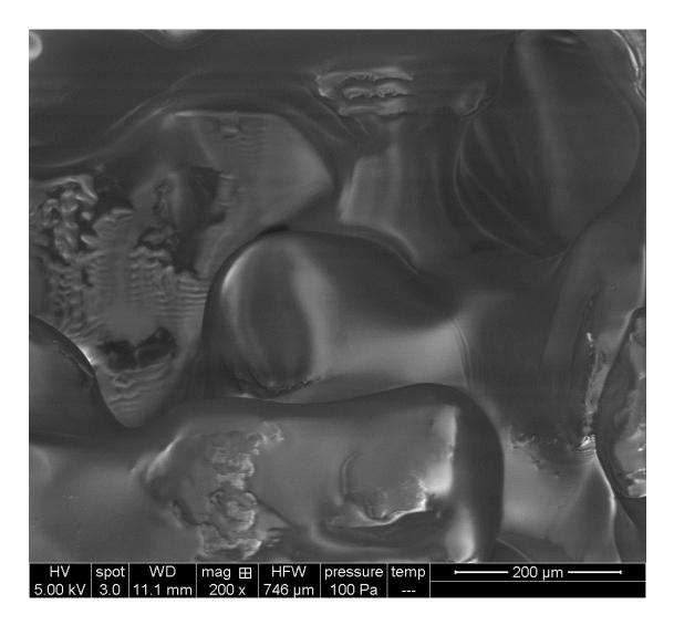
Figure 1: Image of glassy bitumen covering course angular sand grain. The rippling is the result of the electron beam exciting the bitumen
