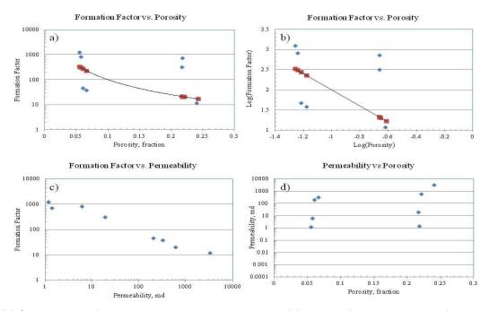
Figure 2: (a) Semi-Log plot for predicted and estimated values of formation factor vs. porosity for all cases. Solid line corresponds to Archie's Law estimation @ m=2 and a=1. (b) Normal scale plot for estimated values of formation factor vs. porosity. (c) Log-Log plot showing the relationship between formation factor and estimated permeability. (d) Semi-Log plot showing the relationship between predicted permeability and calculated porosity for all cases.
