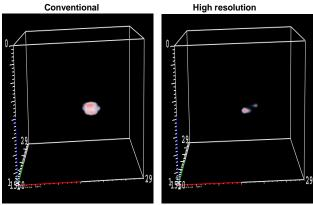
Figure 4. Comparison of 3D stacked volumes from the combined data sets between convention and high-resolution Kirchhoff summation methods.
