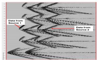
Figure 3. Combination of data sets from the first and second sources in which the data set from the second source had a 0.15 s delay from the first data set.
