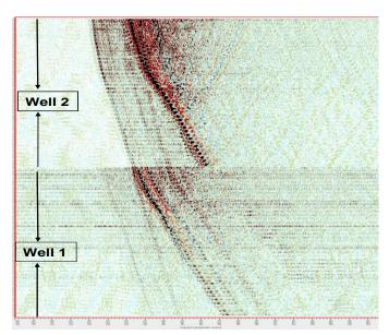
Figure 5. First example of mircoseismic field data recorded by receivers in two observational wells. The event records have a 10 s data length.
