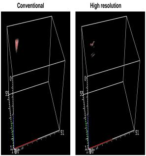
Figure 6. Comparison of 3D stacked volumes from the first field example between convention and highresolution Kirchhoff summation methods.
