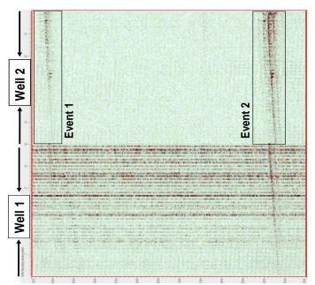
Figure 7. Second example of mircoseismic field data recorded by receivers in two observational wells. The event records have a 10 s data length. Two distinct events are visible on the records.
