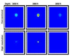
Figure 2. Comparison of stacked images from the first source between convention and high-resolution Kirchhoff summation methods. Star symbol is the theoretical source location.
