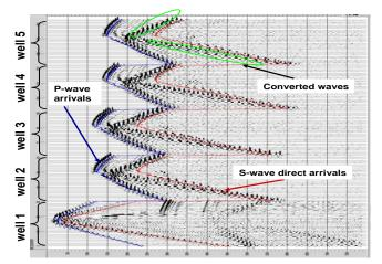
Figure 1 Synthetic data from the first source, showing P- and S-wave direct arrivals as well as converted waves.
