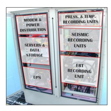
Figure 2: Schematic view of the instrument cabinet located close to the two observation wells at LDA. All instruments can be controlled through the Statoil network to record data throughout the year. In addition to recording instruments, the cabinet is equipped with data servers, an uninterruptible power supply (UPS), air conditioning and more. The arrow in the middle is approximately 1 meter.
