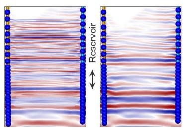
Figure 4 (above): Seismic cross-well section (left) and corresponding section from the 3D VSP baseline acquisition (right). The reservoir interval is approximately 40 m. The two observation wells and permanent three-component geophones can be found along the edges of the two sections.
