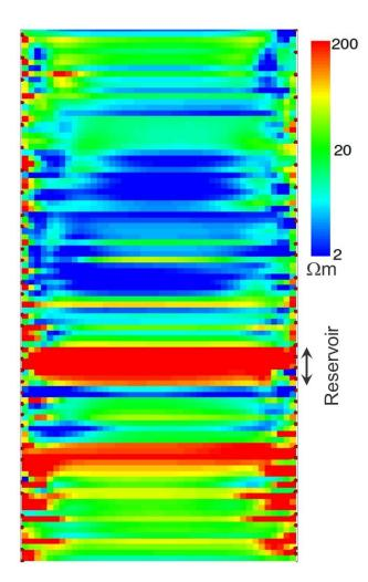
Figure 3 (left): ERT baseline image between the two observation wells. Color scale is in  $\Omega m$ , varying from high (oil sand reservoir and parts of Devonian) to low (mainly water-filled sandstone). Red circles along edges represent ERT electrode locations. The 2D section is 150 m wide and covers a depth interval of approximately 420 m. Noise along well bores is probably due to minor electrical leakages caused by imperfections in the insulation material.
