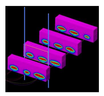
Figure 1: Cross-well experiment layout. Two vertical observation wells (blue) were planned drilled straddling two horizontal production/injection pairs. Distance between producers is 100 meters, while the distance between the observation wells is 150 meters. Color scale represents increasing temperatures during SAGD, warm colors are high temperatures.
