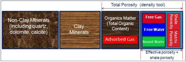
Figure 1: Petrophysical model for shale gas evaluation
