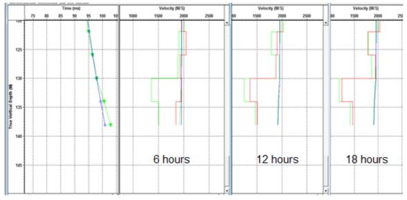
**Figure 6**) arrival times before injection (blue) and after 6h (green); 2) interval velocity before injection (red) and after 6h injection (green); 3) interval velocity after 6h injection (red) and after 12h injection (red); 4) interval velocity after 12h injection (red) and after 18h injection (red).
