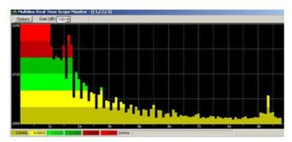
Figure 4) Screen capture of the tool noise levels during the air injection. The injection zone is on the right hand side of the image. The increase noise level from the air can be seen over the bottom tools.
