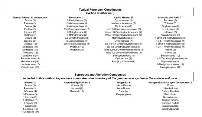
All geochemical samplers were analyzed after the exposure period to the seabed material. Analysis was accomplished using gas chromatography – mass spectrometry (GC/MS), for a range of hydrocarbon compounds from ethane (C2) to octadecane (C18), but also including pristane (C19) and phytane (C20).
