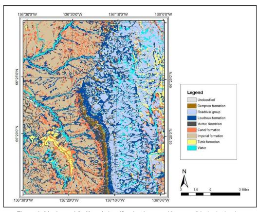
Figure 2. Maximum Likelihood classification image with seven lithological units.
