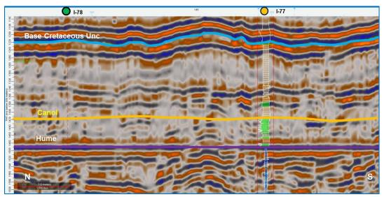
Figure 2. Seismic line flattened on Top Hume showing interpretation of Top Canol oil shale in CMV.
