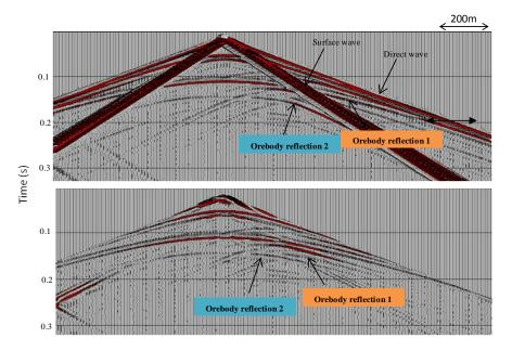
*Figure 2:* (Top) A synthetic seismogram (shot position at x=800m) highlighting the close proximity of the orebody reflections and the source generated noise (Bottom) the same shot record as in (a) with f-k filter applied to surface and direct waves. Some of the orebody reflections are labeled
