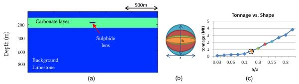
*Figure 1*: (a) Our 2D geological model of a shallow carbonate hosted massive sulphide deposit. (b) Lenses, (h/a <1), and a sphere (h/a=1) showing the end member sizes for an orebody of lateral dimensions 100x100m differing in thickness, h, from 3-100m. (c) Tonnage, calculated using a density of 3840 kg/m<sup>3</sup>, versus shape. The one lens modeled here is represented by the orange lens where h/a= 0.2.
