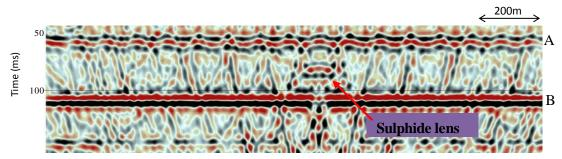
*Figure 4:* The Final migrated section for the 2D sulphide model in Figure 1. Reflector A and B are the top and bottom of the carbonate layer respectively.
