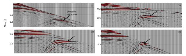
Figure 3: Arrows indicate the positions of orebody reflections for a shot record at x=100m with direct and surface wave energy removed using an f-k filter. (a) without NMO applied, and with NMO correction using a constant velocity of 5000 m/s for (b) no stretch mute, (c) a stretch mute of 90% and (d) a stretch mute of 50%.
