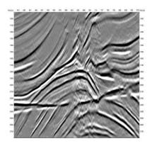
Figure 4b. PSDM image obtained from the ZOMF enhanced gathers. Places of non-hyperbolic traveltime surfaces are deteriorated.
