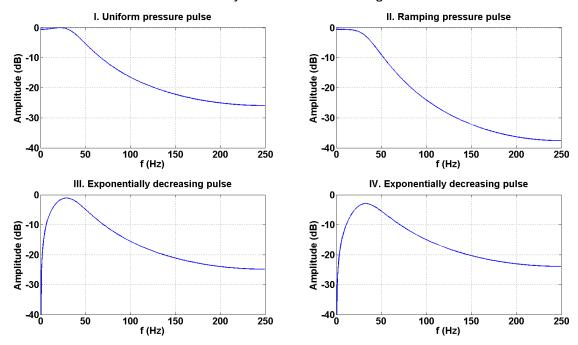
Figure 3: Frequency spectra that result from the displacements shown in Figure 2. In I and II there does not appear to be a low frequency roll-off present in the spectra, however, in III and IV there appears to be a roll-off in frequency below the dominant frequency.
