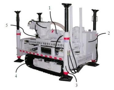
1. Mainframe 2. Power stations3. Support device 4. Crawler bodywork 5. Control panel
