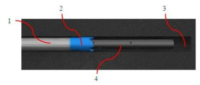
1. Drilling pipe 2. Inner core detachable drill bit 3.Borehole 4. Sieve tube Figure5.Sieve tube borehole protectionsimulation
