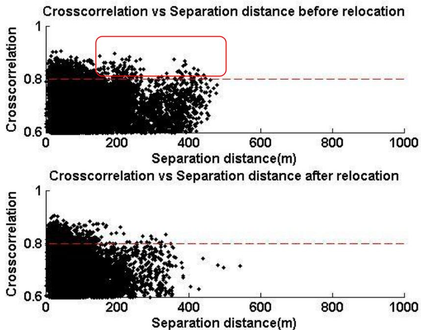
Figure 6: Crosscorrelation coefficient as a function of separation distance before (top) and after (bottom) relocation. Note that after relocation, most doublets separated by larger distances (red rectangle) have been collapsed to shorter distances. This plot can be used as quality controls since doublets with large separation distances suggest location errors due to mispicks.
