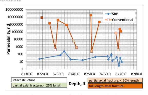
Figure 7: Crushed Permeability and Steady State Permeability Data Patterns
