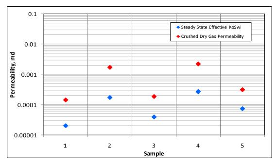
Figure 5: Effective Steady State Oil Permeability vs Crushed Gas Permeability Data Pattern
