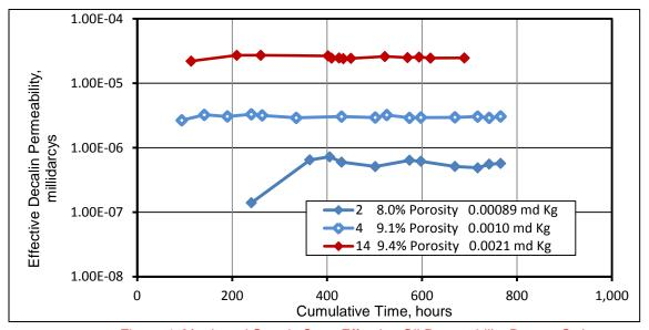
Figure 4: Monitored Steady State Effective Oil Permeability Data at Swi
