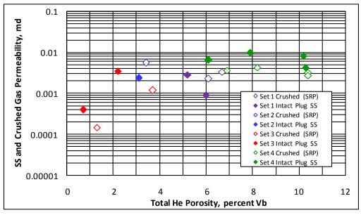
Figure 3: Steady State vs Crushed Gas Permeability Data Pattern
