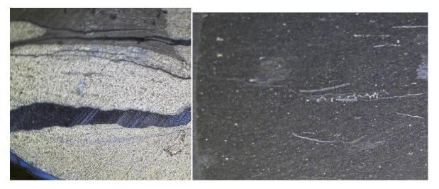
The above photographs show epoxy injected into existing fractures without entry into the surrounding pore structure. Left: a tight gas sand example. Right: a shale sample. Epoxy injection pressure is "matched" to the pore structure: 20 psi was used on the tight gas sand sample and 1000 psi was used on the shale sample.
