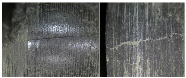
Figure 8: Horizontal Plug Fractures Recorded Using Approximately 200x Magnification
