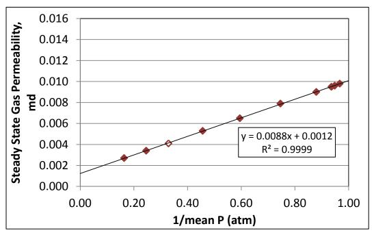
Figure 2: Multi-Point Steady State Klinkenberg Gas Permeability Determination
