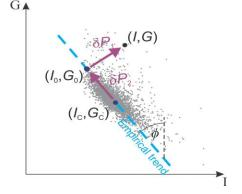
Figure 3: Empirical proxy attributes emphasizing the deviations of AVO parameters along  $(\delta P_1)$  and across the trend line  $(\delta P_2)$ . Grey dots are the measured AVO points
