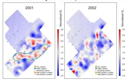
Figure 6: Variations of the calibrated S-wave reflectivity (*I–G*) at Marly for two monitor datasets (labelled). Dashed green line indicates the interpreted area of increased pore pressure.
