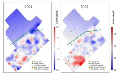
Figure 4: Variations of the calibrated AVO intercepts at Marly reflection for two monitor datasets (labelled). Green dashed line indicates the approximate extent of picked Marly reflection.
