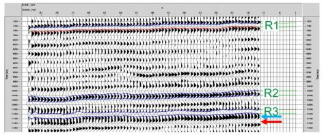
Figure 1: Reference horizons (green labels) used for calibration of reflection and AVA responses. Blue and red arrows indicate the caprock (positive peak) and Marly reservoir (negative trough), respectively.
