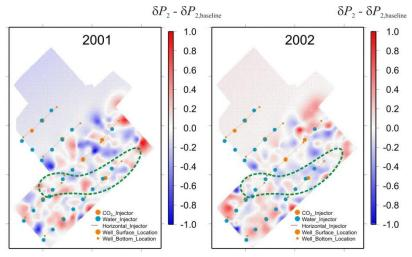
Figure 9: Differential attribute  $\delta P_2$  for Marly reflection. Dashed green lines indicate the interpreted area of increased  $CO_2$  saturation
