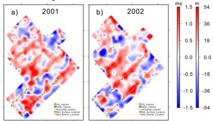
Figure 2: Variations of time differences and thicknessetween the caprock reflector and Bakken (~200ms below caprock):a) 2001 relative to 1999; b) 2002 relative to 1999.
