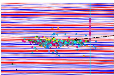
Figure 3: Microseismic events overlaying 3D seismic
