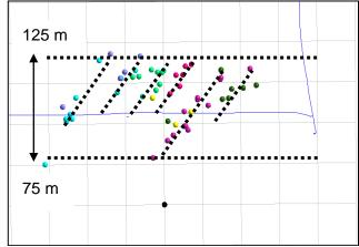
Figure 11: Final representation of the filtered data colored by stage to show a more realistic effective frac growth. Grid scale is 100 meter by 100 meters.
