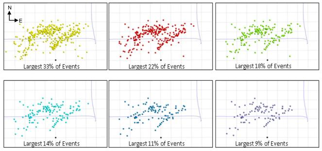
Figure 9: Stepping through event locations as the energy threshold is increased shows event clouds being reduced to linear trends. Grid scale for all images is 100 meter by 100 meters. Treatment wellbore is running East - West with a secondary well running North-South.
