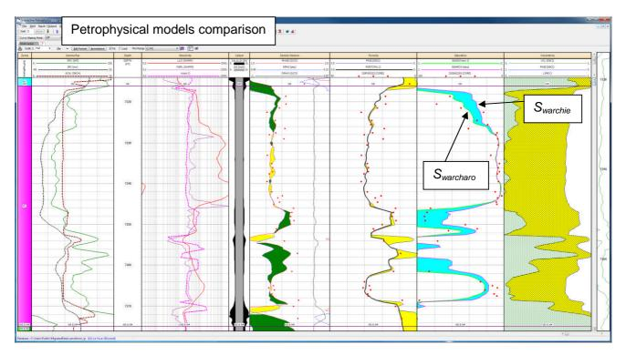
Figure 3: Comparison between the Archie equation results and the Archie-Haro relationships with respect to core data (dots).
