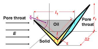
Figure 2: Half pore body upscaled model: Half pore with hydrocarbons (isolator in gray) and water with resistivity  $r_w$  (in yellow) = Half pore full of combined material with equivalent resistivity  $\varnothing r_t$ . Water distribution reflects water-wet conditions. Notice the elongation of the electric path.
