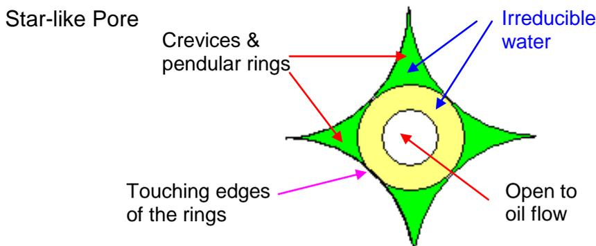
Figure 1: Cross sectional view of a pore: Irreducible water is occupying a space, crevices (green) and films (yellow), that otherwise should be available to non-wetting fluid flow.
