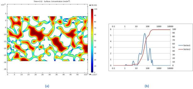
Figure 4: a) surface concentration after t=20 ms. b) Amplitude of the excited protons vs.  $T_2$  series 1, integral of the amplitude vs.  $T_2$  series2.
