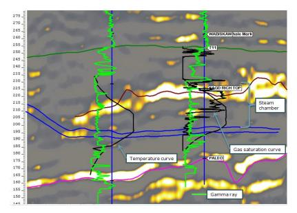
Figure 3 - Producer and injector laterals with developing chamber
