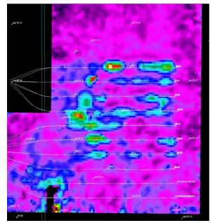
Figure 1 – RMS amplitude difference of 2006 baseline with 2009 monitor surveys
