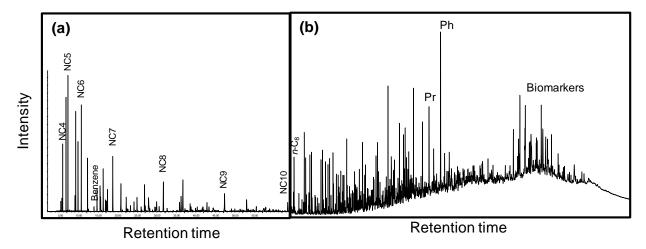
**Figure 1.** Partial reconstructed (a) GC-FID chromatogram of the volatiles captured by Single Drop Vapor Phase Extraction (SDVPE) and (b) total summed ion (60 ions) chromatogram of the total hydrocarbon fraction of a bitumen stained core sample.
