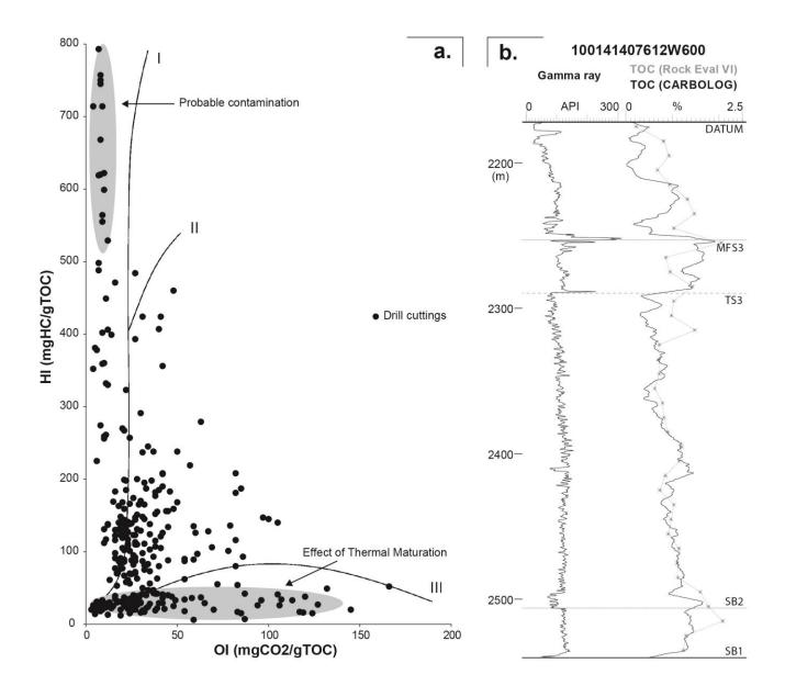
Figure 1: a. Van Krevelen diagram on drill cuttings. b. TOC Estimation with CARBOLOG.
