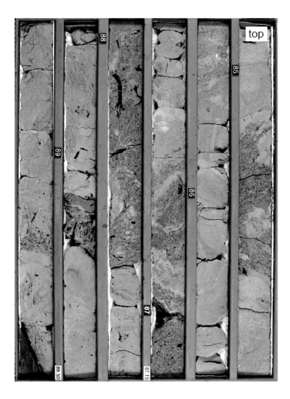
**Figure 2.** Sand dikes developed as numerous intertwined conduits that mobilized fluidized sand upward, often mixed with wall rock. Mud laminar mud ribbons were usually suspended in the flow. Each core box slat is 75 cm long.
