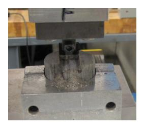
Figure 2, Sample plug on a mechanical scratch tester
