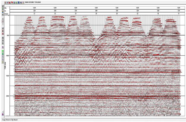
Figure 2 - Single vibrator, single sweep, 3D stack (Single vibrator, 1 sweep per VP at 8.3m)
