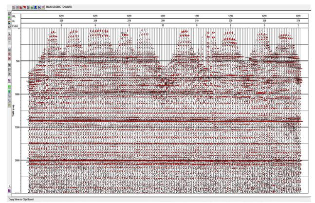
Figure 3 - Production shots equivalent to Figure 2 (3 vibrators per fleet, 1 sweep per VP at 25m)
