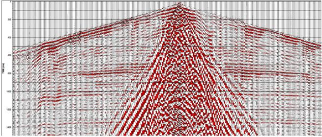
Figure 4 - Receiver gather, Eastern Alberta – Mini-vibrator, single sweep per VP (T<sup>2</sup> gain function only)
