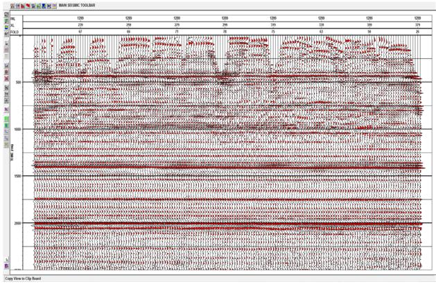
Figure 1 - Full fold 3D stack - production data (3 vibrators per fleet, 1 sweep per VP at 25m)
