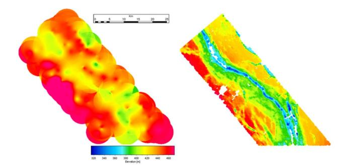
Fig 2: Elevation of bedrock (shale), from borehole data only (left) and from accurately processed and modelled AEM data (right) and boreholes (adapted from Sapia et al., 2014).
