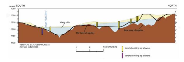
**Fig. 3** Hydrogeological section provided by the AEM survey. The columns show the boreholes with stratigraphic info, the black line represent the bottom of the aquifer based only on the boreholes. Notice the greater thickness of the aquifer on the right side, on the contrary of what expected (Courtesy: USGS Scientific Investigation Report: 2011-5219).
