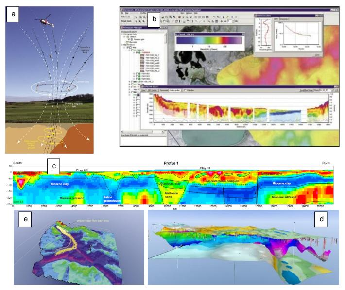
**Fig. 1** Schematic of workflow applied in Denmark for groundwater mapping. a) data acquisition, b) data processing and inversion to produce 3D resistivity model, c) geological conceptualization of resistivity model, d) geological model, e) flow model
