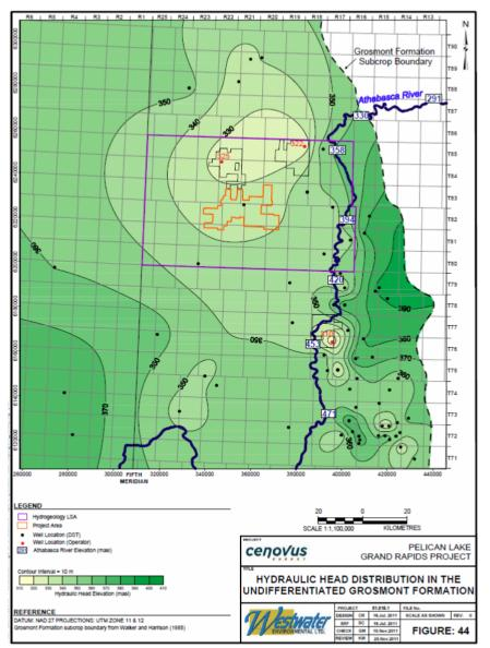
Figure 1 . Hydraulic head distribution in the undifferentiated Grosmont formation. From Cenovus, 2011, Volume 4, Appendix 4-IV, Figure 44.
