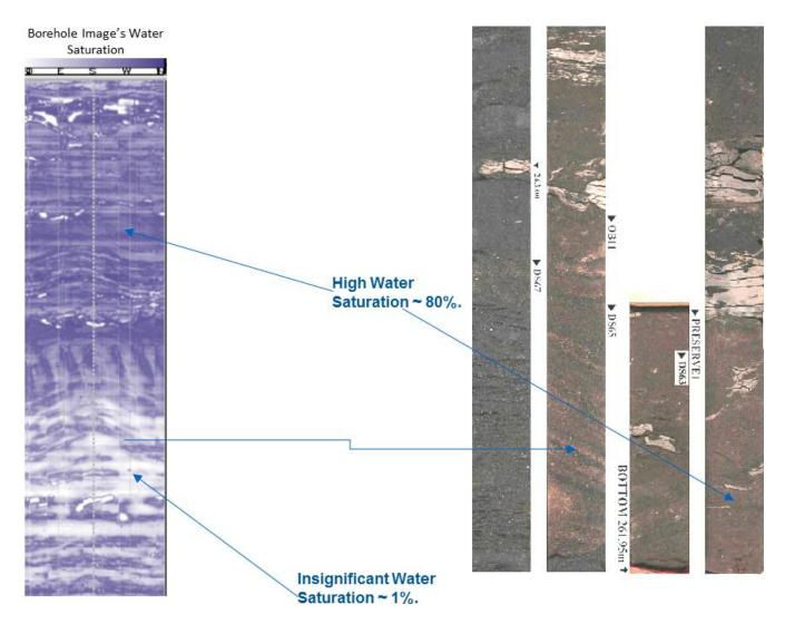
This method assumes that the borehole resistivity measurement responds mainly to clay and water content. The grain size, shape and sorting effects are assumed negligible. The comparison between the Dean-Stark tests and the borehole image derived water saturation will be presented.
