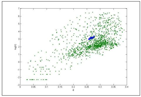
Figure 1 – Porosity vs permeability distributions (original and scaled up)
