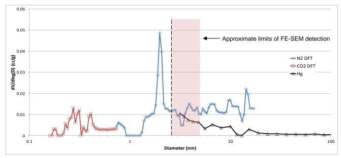
**Figure 2.** Mercury pore throat distributions combined with nitrogen and carbon dioxide pore volume distributions. Where mercury and nitrogen pore sizes overlap, mercury measures pore throats while nitrogen measures pore volume which leads to some discrepancy in measured volume.
