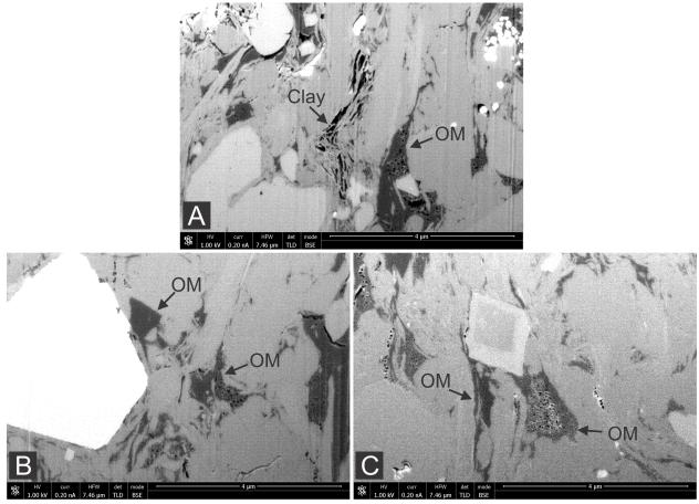
**Figure 1.** *A*. Highest maturity sample ( $T_{max}$ : ~480) showing variably developed organic matter porosity and porosity associated with clays. *B*. Middle maturity sample ( $T_{max}$ : ~469) showing variably developed organic matter porosity. *C*. Lowest maturity sample ( $T_{max}$ : ~445) showing some porosity associated with organic matter.
