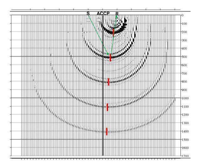
Figure 1. Nonzero offset trace response of the 3D shot profile WEM of converted waves. The red picks show the CCP at the bottom of the migration ellipses. The green arrows show the downward going P-wave of the source and upward going converted S-wave to the receiver. The asymmetric amplitude response is natural to shot profile migration.
