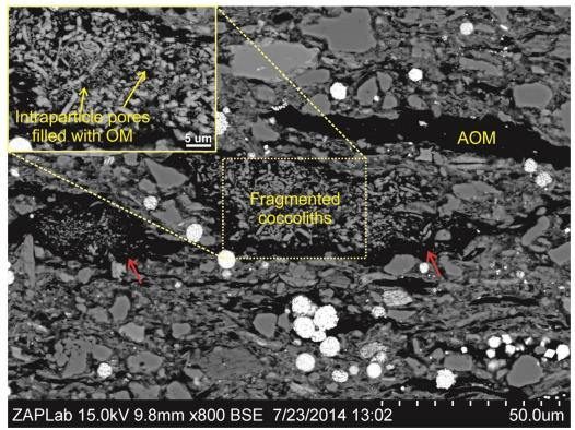
Figure 1: Backscatter scanning electron photomicrograph of a vertical section of mudstone of the Puskwaskau Formation, north-central Alberta. Amorphous organic matter (AOM) and framboidal and euhedral pyrite is ubiquitous in this sample. Fecal pellets (red arrows) contain fragmented coccoliths and display considerable porosity. Intraparticle pores contain abundant organic matter (OM).
