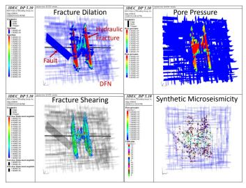
**Figure 4.** Geomechanical modeling results of Case 1. Upper left: the fracture dilation or opening. Upper right: the pore pressure contours. Lower left: the shear displacements contours. Lower right: the estimated synthetic microseismicity.
