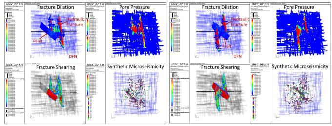
Figure 5. Results of Case 2 (left) and 3 (right).
