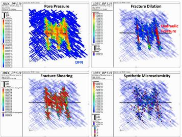
**Figure 1.** Geomechanical simulation of a hydraulic fracture network. Upper left shows the simulated pore pressure diffusion within a DFN (blue). Upper right shows the fracture dilation or opening of the primary hydraulic fractures (red segments). Lower left shows the calculated shear displacements, indicating the induced slip within the DFN. Lower right shows the estimated microseismicity.
