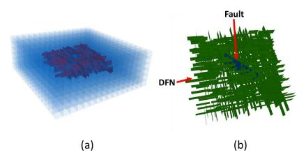
Figure 3. a) Geomechanical model with faulted region in center. b) Fault region (blue) and DFN (green).
