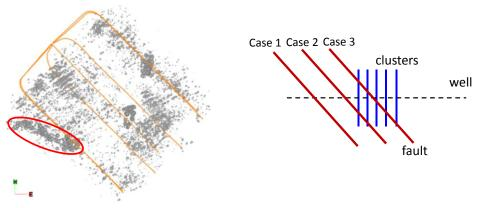
**Figure 2.** Microseismic monitoring of HRB hydraulic fracture (left) showing an example of fault activation (red oval, after Snelling and de Groot, 2014). Schematic of geomechanical model (right) showing three cases of a fault crossing the well at different positions relative to five perforation clusters.
