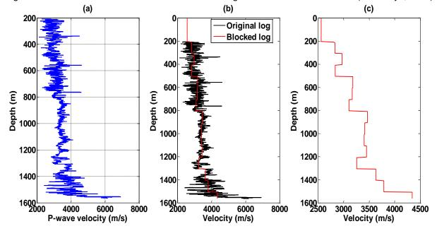
Figure 2: (a) Well 12-27 P-wave sonic log; (b) shows the original log in black and the blocked log in red; (c) shows only the blocked log. The depth step of the log being blocked is 100m.
