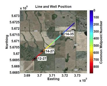
Figure 1: The 4.5km Hussar seismic line is shown along with the locations of 3 wells (from Lloyd, 2013).
