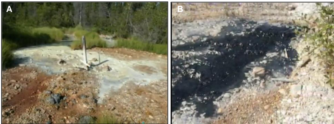
Figure 4: Discharge of sulphurous water (Fig. 4A) and metal-containing saline water (Fig. 4B: a cold 'black smoker') from artesian open boreholes located close to each other in the area of the X-15 ore body. Flow from borehole on Fig 4B estimated to be 1-2 litres/sec. (Source: YouTube video "Pine Point Mine: History in the Landscape": http://www.youtube.com/watch?v=DgY6biryzQc )
